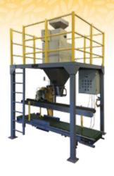
This type of machine is designed for packing materials with good fluidity into open mouth bags. Rice, Seed, Urea, Compound Fertilizer, Granulated Sugar, Rubber Granule, Feed, Fertilizer, Granulated PVC, Active Carbon, Construction Materials, Refractory Material, etc.
