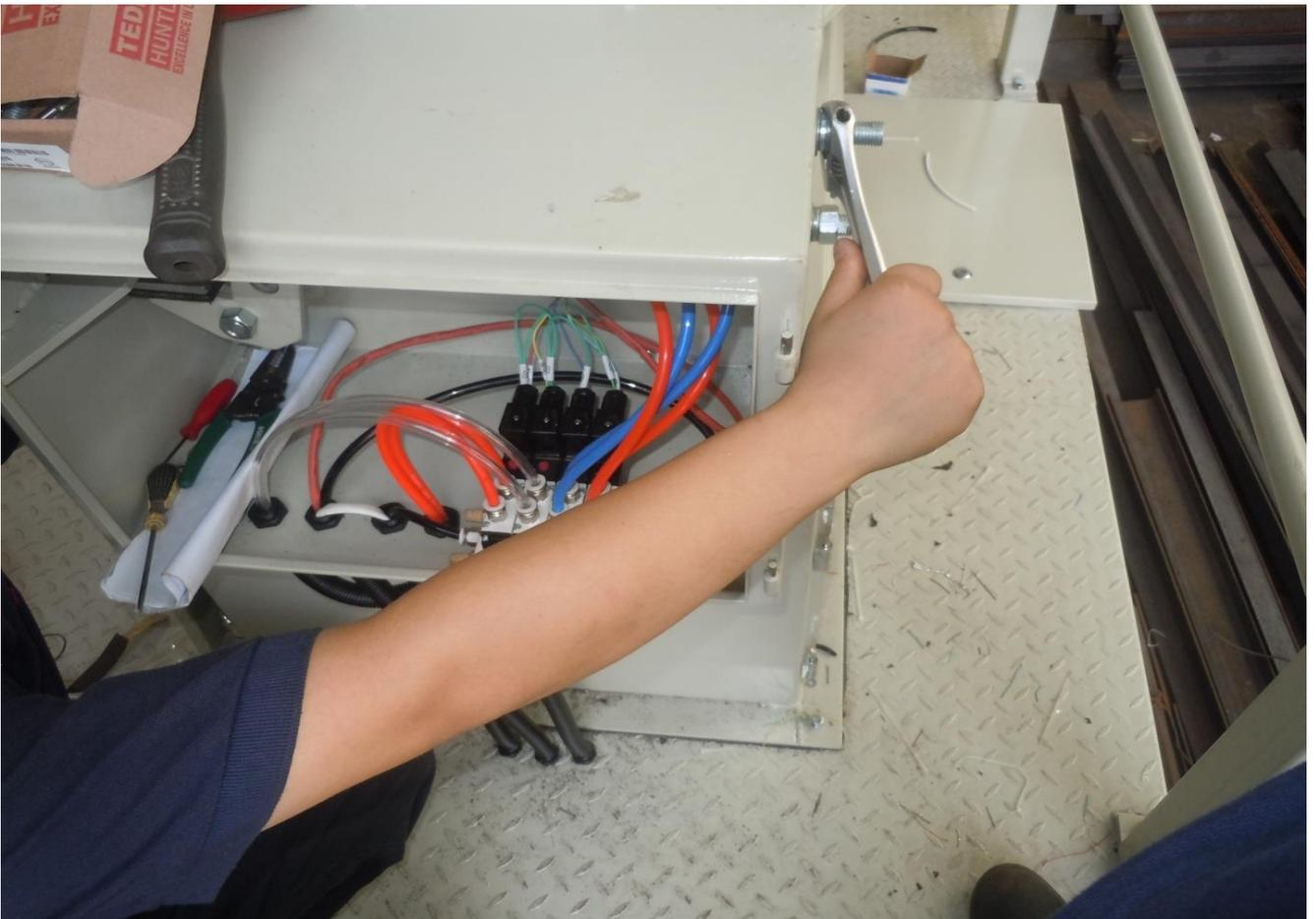
**Make the** air cylinder move to the end, check the size of the small feeding mouth when operating, Notice the size can not too big.( as the below picture)
